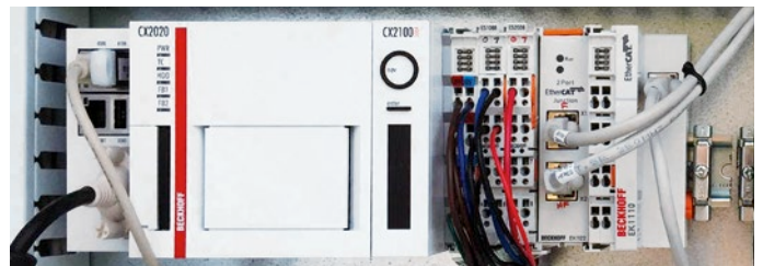
A CX2020 Embedded PC with TwinCAT NC I software serves as integrated control platform for PLC and motion control.
