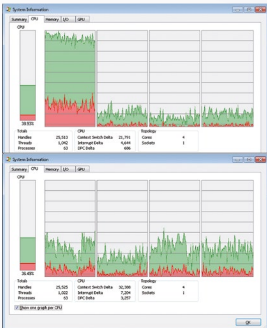
Fig. 4: CPU load; top: graphics load on one core, bottom: graphics load distributed across all four cores
